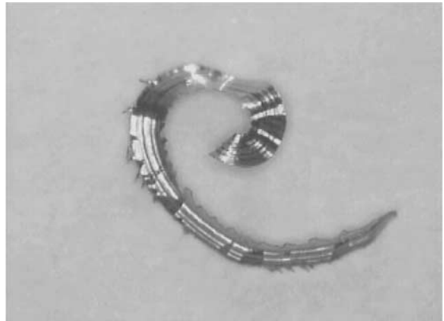
Fig. 17. The high-pressure chip shape at 40 HRC for a coated insert.
