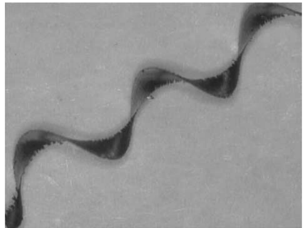
Fig. 10. The conventional coolant chip shape at 35 HRC for an uncoated insert.
