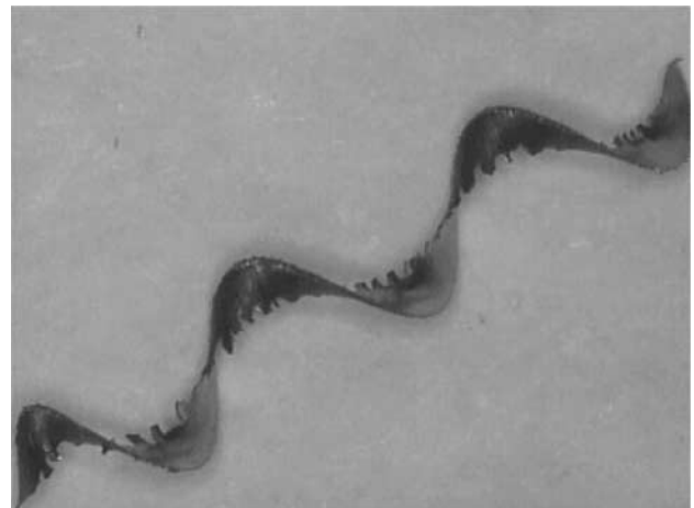
Fig. 11. The high-pressure chip shape at 35 HRC for an uncoated insert.
