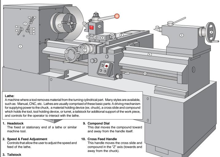
That part of a machine tool. such as a lathe or cylindrical grinder which supports the end of a workpiece with a center. It may be positioned at any point along the way of the bed, and may be offset from center to machine tapers.
