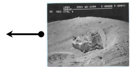
This is an important practical point -- if crystal retention is not limiting bit or blade performance, a coated diamond will not provide any advantage.
