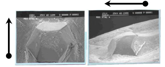
There is no gap between bond and crystal, particularly at the contact/leading edge. The bond tail at the trailing edge is smooth and un-eroded.
