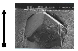
The bond is clearly deadhered from the crystal at the most critical leading edge. There is also deep erosive damage. The bond tail is also not well formed. Not surprisingly, the crystal is showing deep fracture damage at the trailing edge where reflected tensile strain is highest. Bond retention in this case is limiting tool life.
