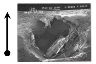
The crystal is gone, leaving an empty pocket in the bond. There is diamond wear debris in the pocket indicating that crystal failure occurs prior to, or concurrent with, popout and there is weak adhesion diamond-matrix with this bond. The bond tail is gone as well. There is no protruding crystal to protect the bond from the hard stone work piece and abrasive debris. Tool life suffers accordingly.
